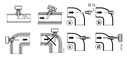
NOTICE! For sensors with non-sealing threaded nipples G  $\frac{1}{2}$ , sealing means must be used with the threaded connection (e.g., hemp, Teflon tape or similar).
