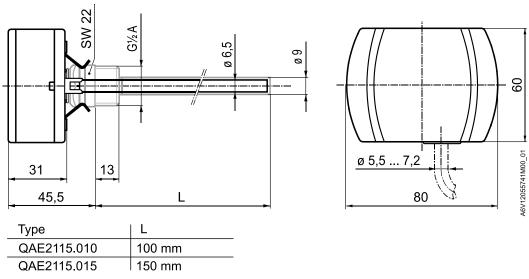
Variable immersion length: with accessory AQE2102 Accessory compression fitting **AQE2102**
